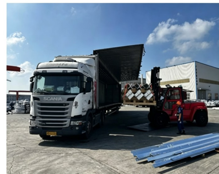
Operation site of the wing van. Wing doors are fully opened, and overlength pallets are smoothly loaded and unloaded from the.
