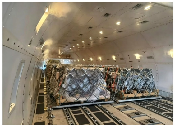
Inside the main cargo hold. Pallets are secured sequentially on the roller floor, awaiting door closure.
