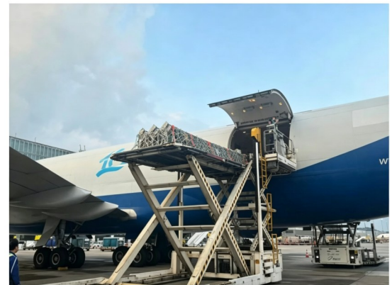
▲ Hong Kong Airport, Boeing 747-8F side door loading operation. The main cargo side door is fully opened. The high loader
